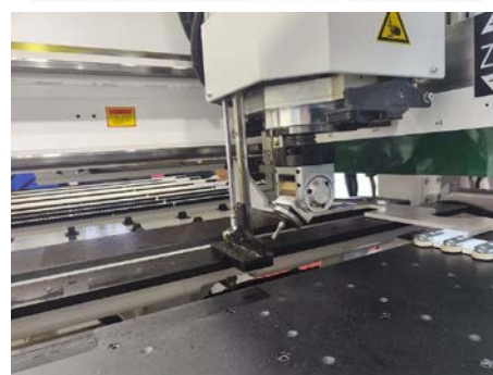
2-position in-line tool magazine Automatic tool changing spindle (with C-axis) High speed drilling block Automatic tool changing spindle 8-position in-line tool magazine
